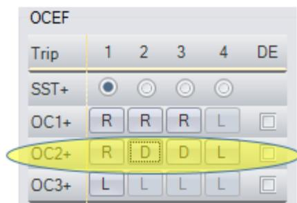
Figure 3: OC2 and Disable Fast Trips (DFT)
