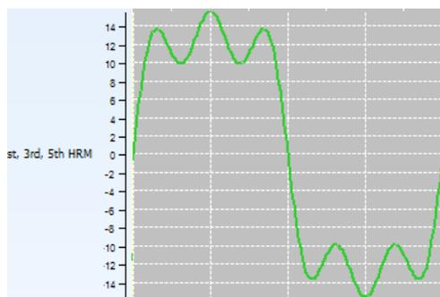
Figure 4: A Waveform with High Harmonic Content
